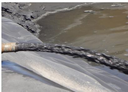
Inlet water to the separator contains minerals with c:a 18% concentration and density 3,5.
