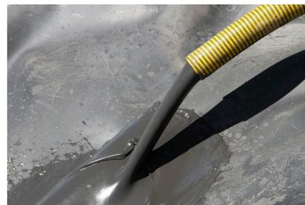
Outlet of sediment from separator with about 80-90% concentration\*).
